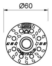
Marking of the anchor sleeve: Anchor type (Combi Fix Plus) Use category A,B,C,D, E
