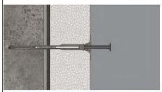
Place the anchor into the drill hole. The bottom side of the plate must be flush with the ETICS.
