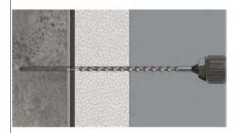
Drill the hole perpendicular to the substrate surface. Clean the drill hole 3x.
